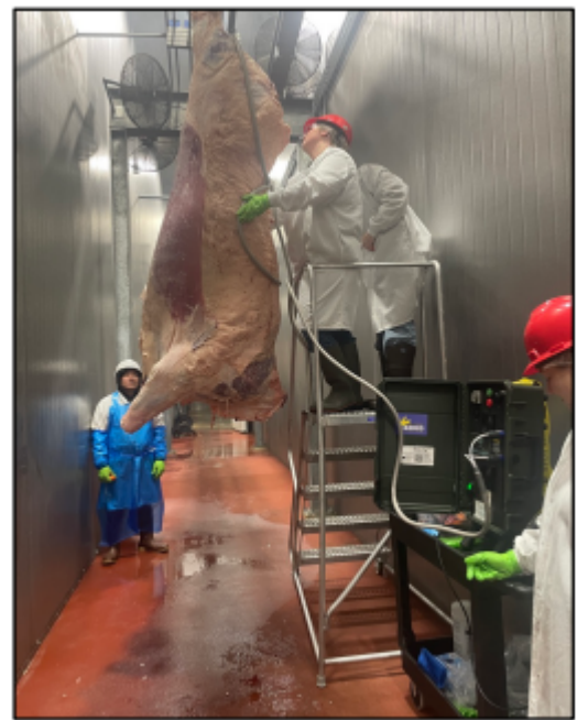
Image 1: Application of PEMF treatment to a beef carcass
